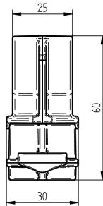
Adapter with "snap-on" for roof conductor holder PR-ÖKO 2 for mounting the HVC-85 on flat roofs
